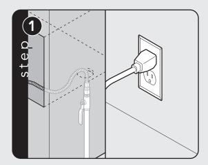
Connect gas and electrical. Before placing appliance in operation, always check for gas leaks. This must be performed by your dealer, a qualified licensed plumber, or gas service company.
